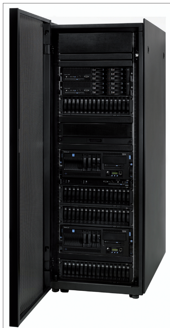
Figure 1: A typical DAS system, the RDL-AS42S3, with 42 disk bays in a four-height-unit-tall case.
