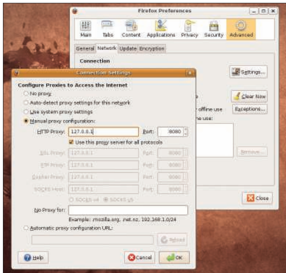
Figure 1: To point Firefox to Ratproxy, first select Edit | Settings in the main menu; select Advanced , choose the Network tab, and click on the Settings button. In the Connection Settings dialog box, enable Manual proxy configuration , and type the settings for the proxy configuration.
