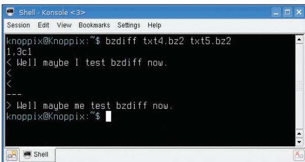
**Figure 2: With zdiff or bzdiff, you can easily find differences between different versions of compressed files.**
