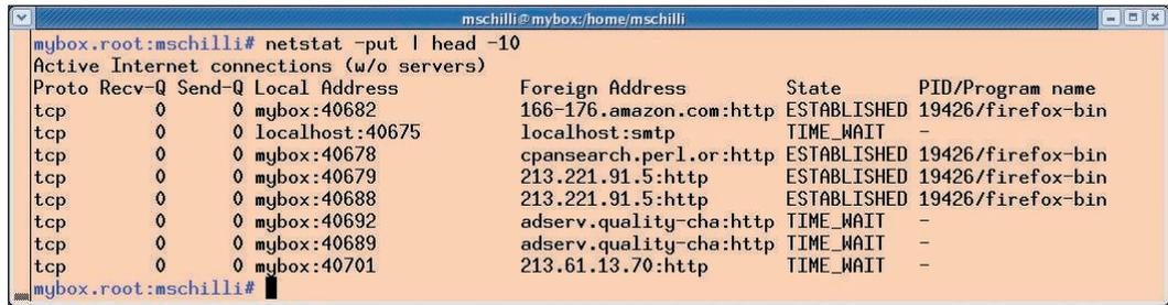
Figure 2: The output of the netstat -put command shows a list of all active TCP ports.
