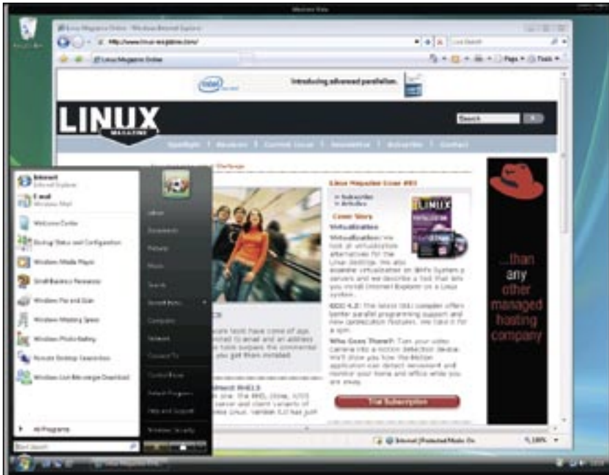
Figure 1: Appearances can deceive: This is not a picture of a Vista system. What you see is Rdesktop displaying Windows in full screen mode on Linux.
