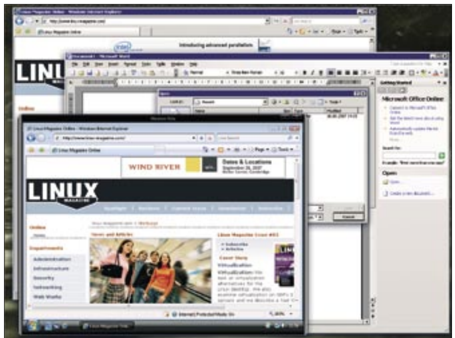
Figure 2: SeamlessRDP lets you display individual Windows applications on the Linux desktop.
