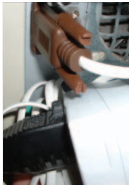
Figure 5: The X10 control unit with a serial connector can send signals from the computer to the control unit over power cables.
