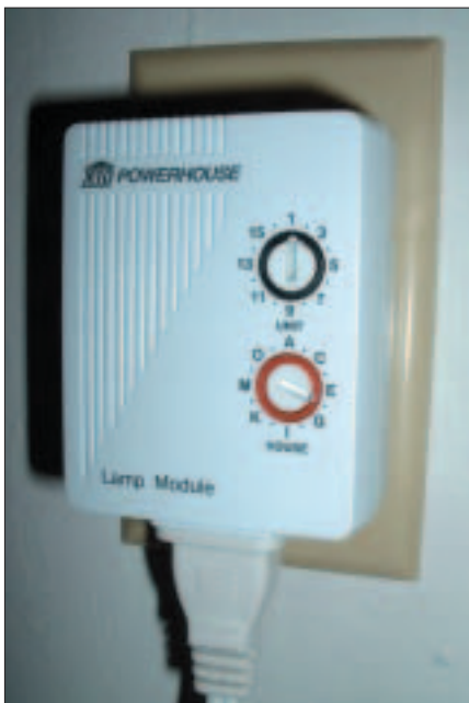
Figure 4: The X10 control unit waits for signals and switches the power on or off.
