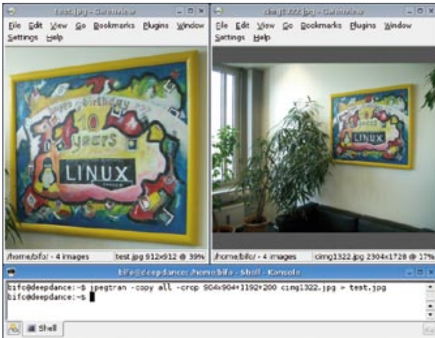
Figure 3: Jpegtran supports loss free image cropping. If the selection to be cropped does not sit exactly on a JPEG block border, Jpegtran scales the selection by the required number of pixels.
