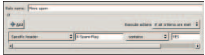
Figure 4: A filtering rule that checks all messages that have the X-Spam-Flag set to YES in the header.
