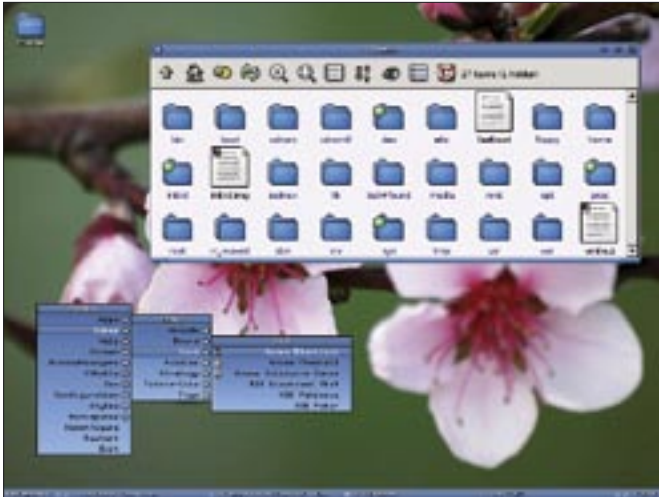
Figure 5: Zen Linux comes with the Fluxbox window manager and the ROX file manager.
