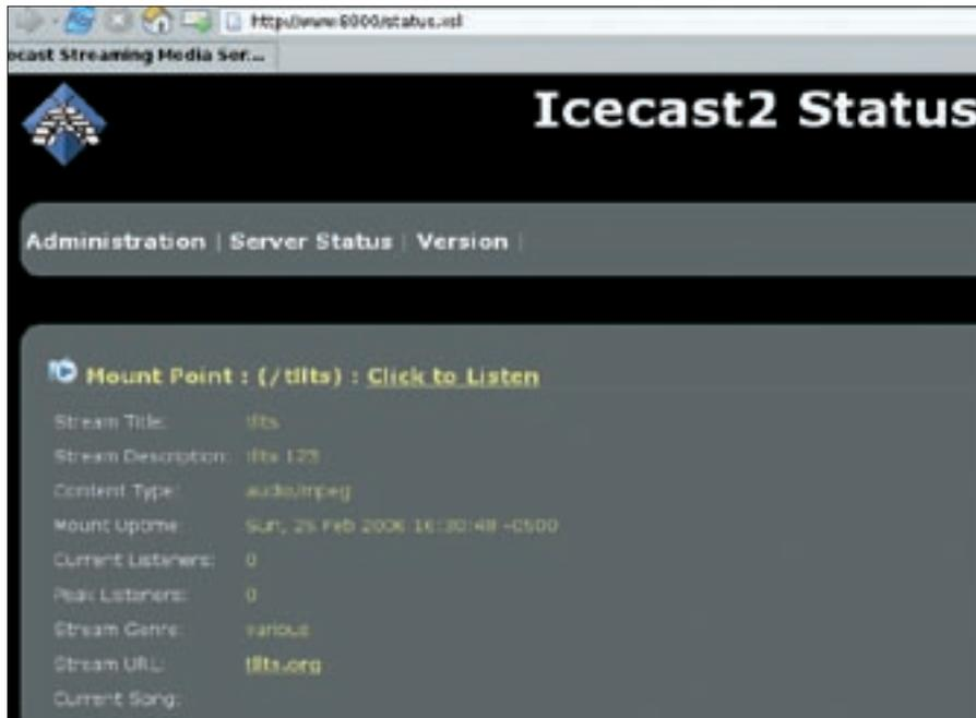
**Figure 3:** The general information page of the Icecast web interface displays information about the mount-points and allows clients to easily connect.
