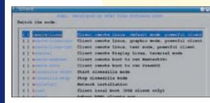
diskless client machines. Similar to the Linux Terminal Server Project (LTSP), it uses a Pre-Boot Execution Environment (PXE) to allow workstations to boot from a server on a network prior to booting the operating system on the local hard drive. DRBL uses NFS to let clients authenticate, and share files and directories over a network. This approach means that DRBL can support more clients (usually 30 to 40) per server than LTSP (usually 20 to 30 clients).
