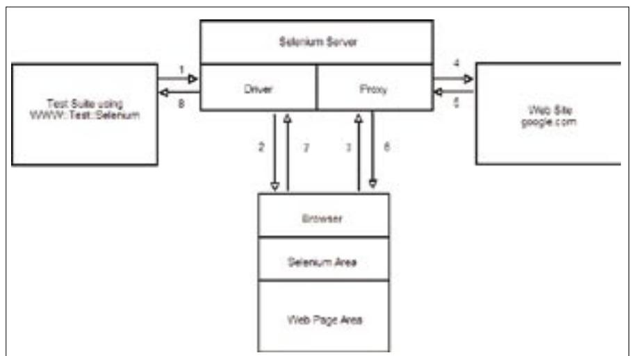
**Figure 5:** The test script talks to the Selenium server, which in turn remote-controls to the browser. Selenium's proxy server manipulates the browser's communication with the website.
