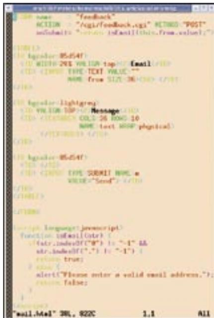
Figure 2: Use HTML with JavaScript to check if a typed email address can be accepted.
