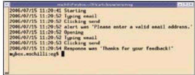
Figure 3: The `emailcheck` test script uses Selenium to control a Firefox browser session. It simulates the input of an invalid and a valid email address and outputs both the content of the resulting error dialog and the successful server response.
