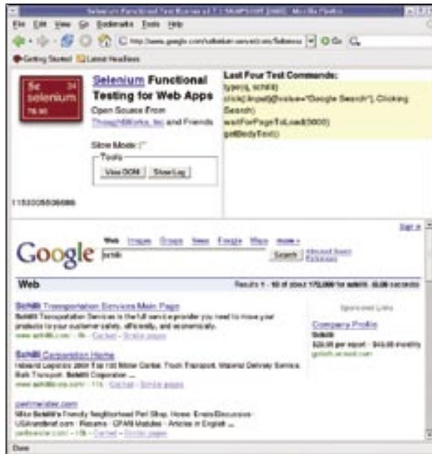
**Figure 4:** For its tests, Selenium sets up its own browser profile. It then tells the browser to surf to a page, while showing the remote control features in the top half of the window.
