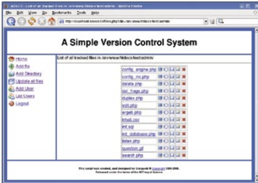
Figure 3: Lightweight version control: ASCVS provides simple version control on any PHP-capable web server.
