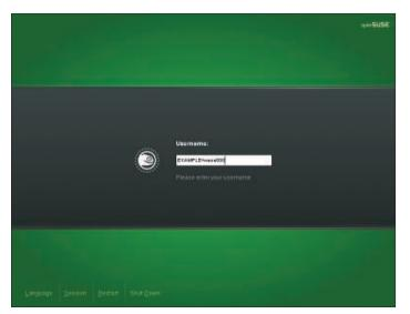
Figure 5: The GDM display manager requests a login name on authentication. In this AD, the name consists of the domain name, EXAMPLE, a plus sign as a separator, and the username.
