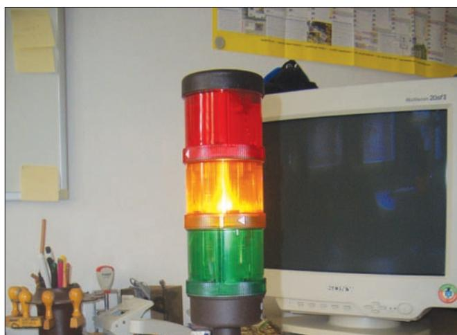
Figure 2: This hard-to-miss traffic light on the admin's desktop warns the admin of trouble on the network - the greener the screen, the healthier your network is feeling.
