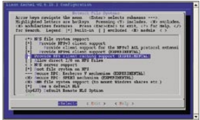
Figure 3: The highlighted options enable the cache for NFS.
