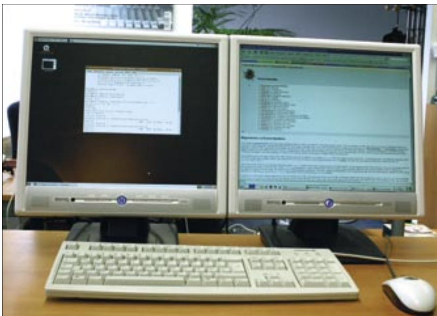
Figure 2: The two displays are connected to two different machines. Thanks to X2X or Synergy, a single mouse and keyboard are all you need. The approach is similar to a Cinerama configuration.
