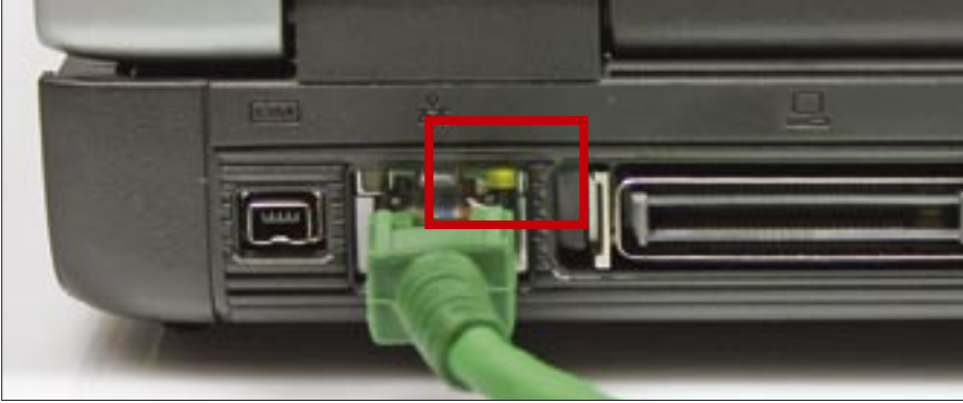
Figure 2: If the network device has been disabled via ifconfig or ifdown , the link LED may be lit when a cable is attached, however, the driver will not attempt to detect the network speed, or report that a cable has been plugged in.
