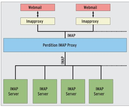
Figure 1: While Perdition is a full-solution IMAP and POP proxy, Imapproxy mainly helps to accelerate webmailers by providing a local IMAP connection cache.
