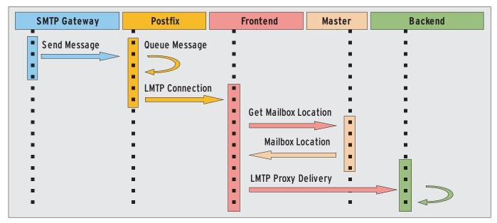
Figure 2: The mail gateway delivers the incoming message to the SMTP server. The SMTP server uses LMTP to forward the message to the front-end server, and finally the message is delivered to the matching back end.
