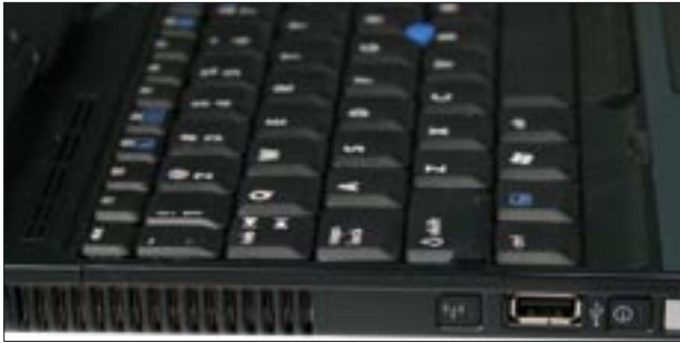
Figure 2: The button with the antenna symbol on the left of the USB connector disables and re-enables WLAN and Bluetooth without rebooting the system. The info button between the power switch and the USB connector produces a scan code and will start the Gnome help browser by default.
