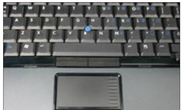
Figure 3: HP equips the NC4200 with both a track point and a touchpad, supporting users with the two most preferred mouse replacements. The grooved area on the right side of the touchpad works as a scrolling wheel and third mouse button.
