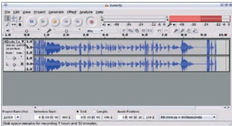
Figure 4: The meter in the upper right corner of the Audacity main window dances to show you how loud your voice is.
