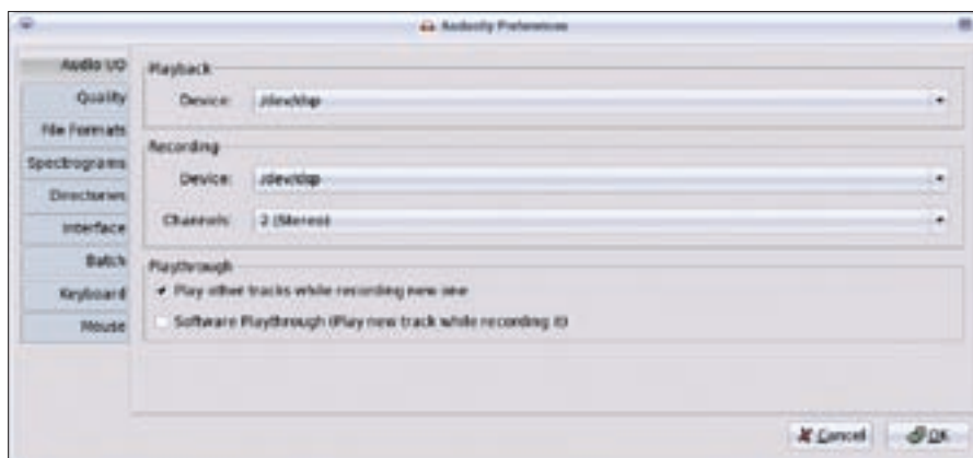
Figure 2: Configure playback, recording, and playthrough settings in the Audacity Preferences dialog box.
