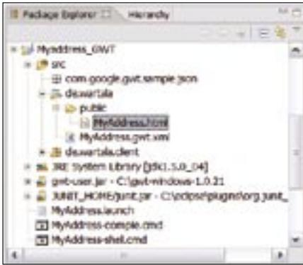
Figure 3: The Google Web Toolkit can optionally create Eclipse project files, giving programmers the ability to import them into the IDE as a project.
