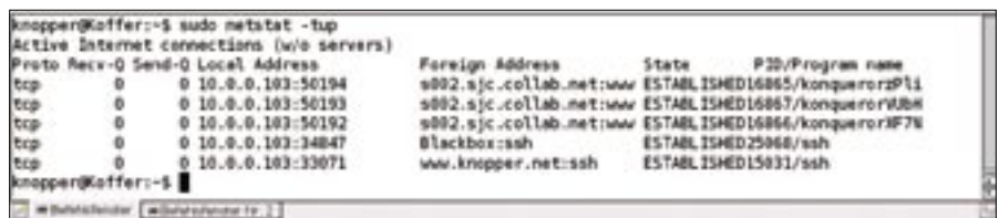
Figure 2: netstat -tup identifies your client connections.
