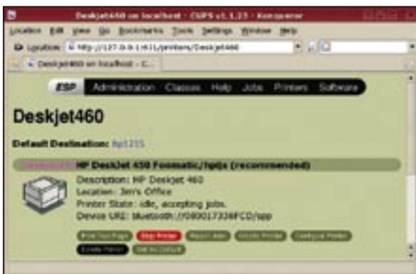
Figure 3: The completed Bluetooth printer configuration.
