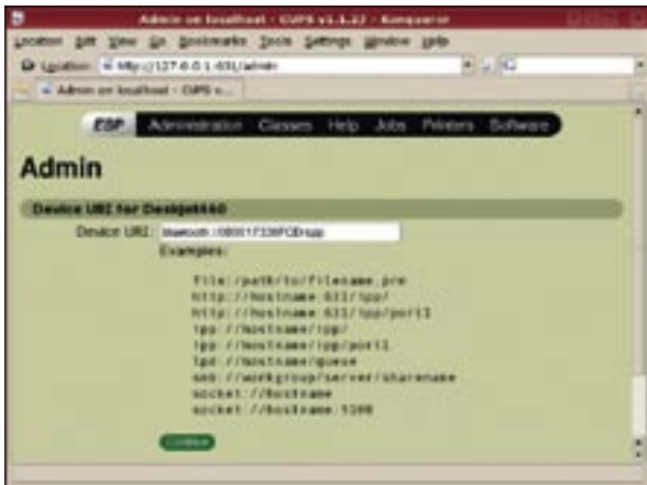
Figure 2: Configuring the Device URI to connect to a Bluetooth printer.
