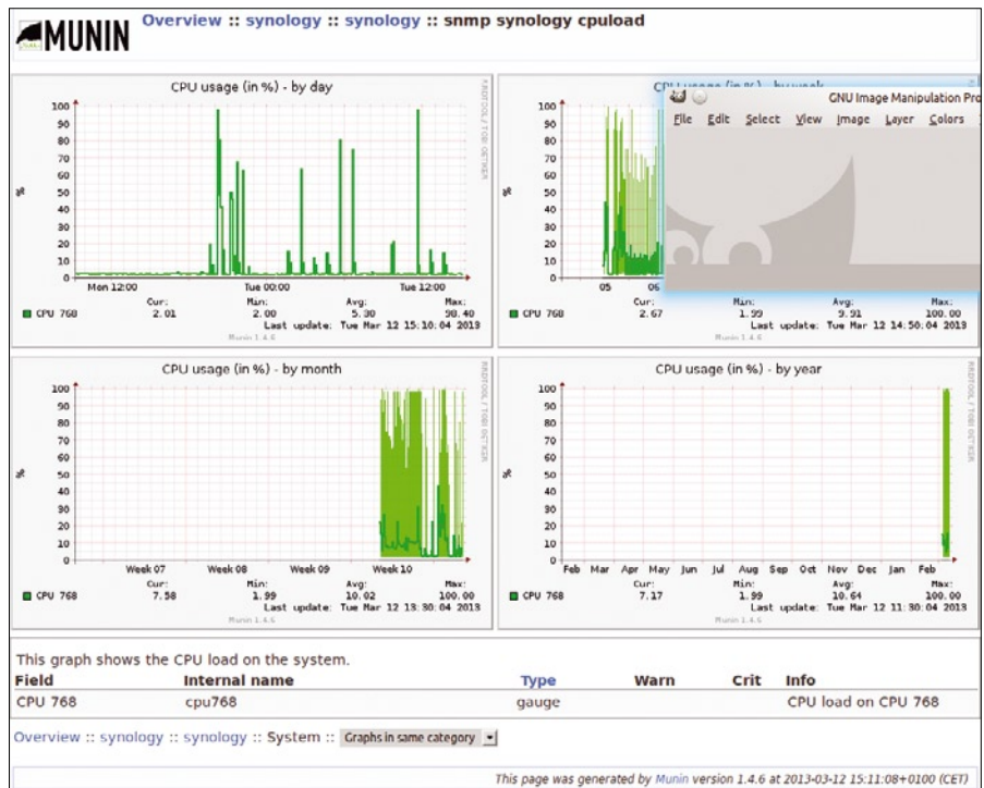
Figure 1: Shortly after the successful SNMP setup, the first data starts to reach RRD databases.
