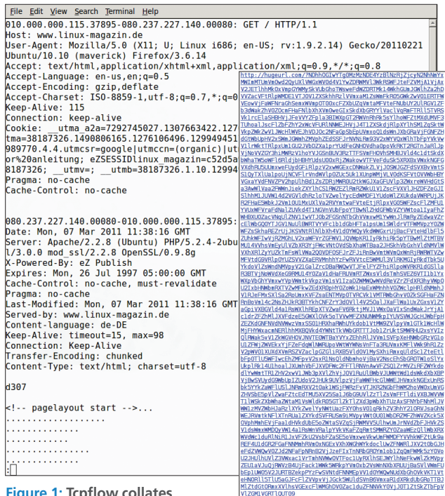
Figure 1: Tcpcflow collates packet dumps from the client (top left) and the server (bottom left) to create flows. The right-hand image shows one huge URL from HugeURL.com.
