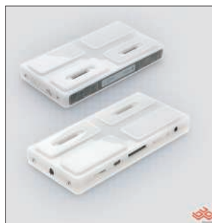
Figure 2: BUGbase is the basis of a modular system that allows users to design their own hardware.
