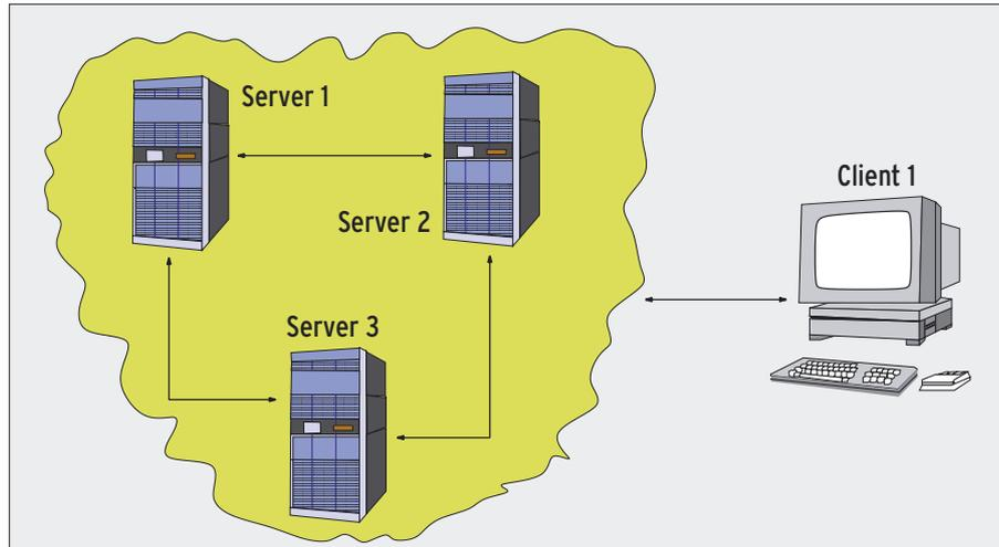
**Figure 3:** The three NTP servers (on the left) are running in symmetric mode and acting as redundant, mutual time sources. The client (on the right) simply polls one of the servers for the correct time.
