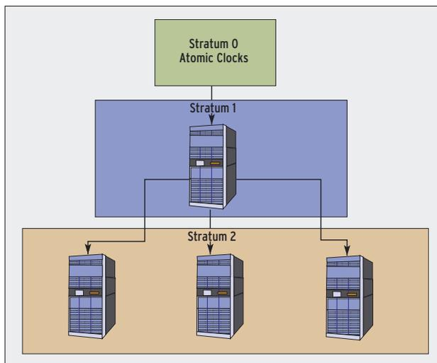
**Figure 2:** An NTP network is organized hierarchically in multiple levels. Time sources such as atomic clocks reside in stratum 0; computers that reference this kind of clock directly reside in stratum 1. In turn, they provide stratum 2 computers with an accurate time signal.
