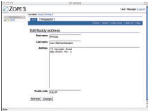
Figure 1: This editing form was generated automatically by reference to the data schema for the content component.
