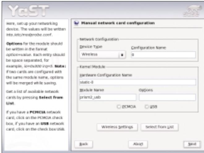
Figure 1: Setting up a USB WLAN adapter with Prism2 chipset on SuSE Linux 9.1.
