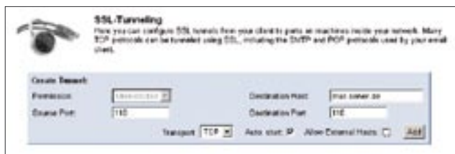
Figure 4: SSL-Explorer provides a simple dialog box for creating a tunnel from the client to ports on other computers.
