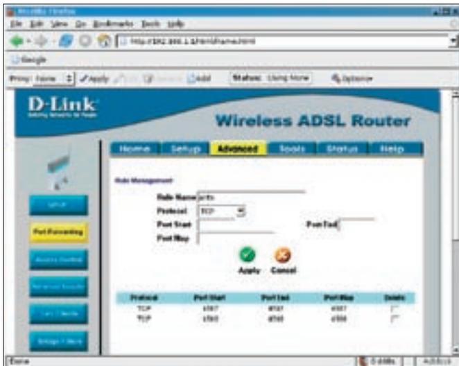
Figure 2: Port forwarding for routers is commonly configured via a browser interface.
