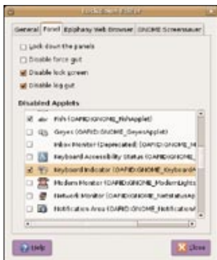
Figure 1: The Pessulus lockdown editor enables GConf keys that deny specific Gnome functions to users.
