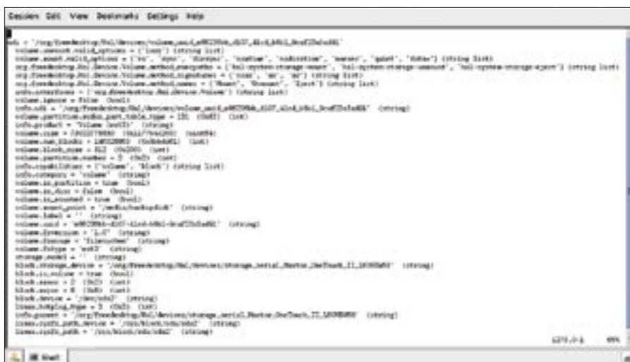
Figure 1: The `shals` command outputs all devices and properties registered with the Hardware Abstraction Layer (HAL).
